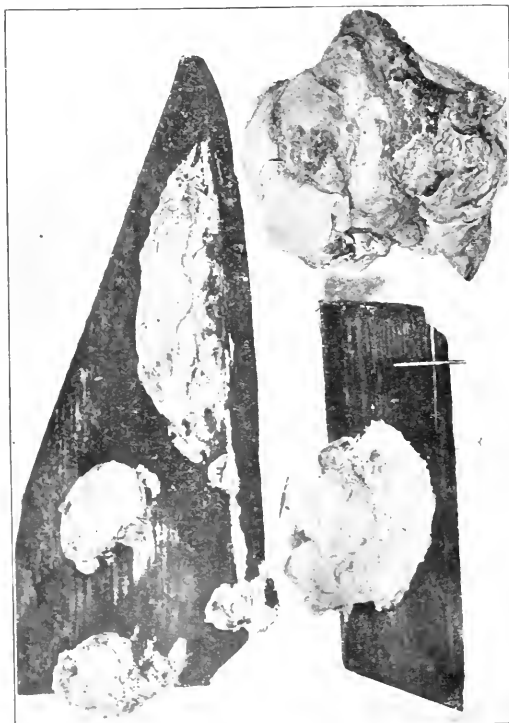
Fig. 4.—White, irregular, lump-like fruiting-bodies of Fomes officinalis found growing in beams in a weaved roof. ( \frac{1}{2} actual size.)
